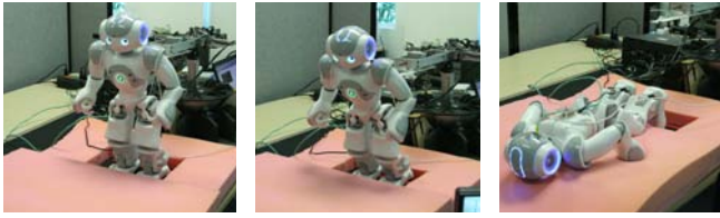
Fig. 7. Default case: without direction-changing fall controller, the NAO robot, when pushed from behind by a linear actuator, falls forward.
