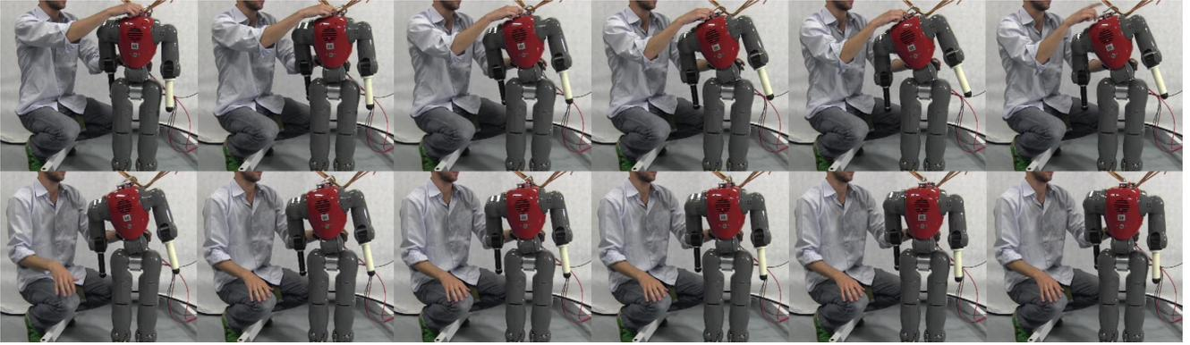
Fig. 7. Snapshots from the video of the experimental validation of the WBMC with the COMAN robot (taken at  $2Hz$ ). In this instance the robot configuration is perturbed by forcing the waist roll joint to change its angle. As the robot is released the *MinEff* brings the robot back to a vertical, minimum effort configuration. The resulting motion is damped by the *MomJ* attractor, that prevents the velocity to grow uncontrolled.
